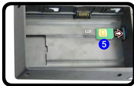
Figure 1 - 18 USIM Card & Battery Insertion
