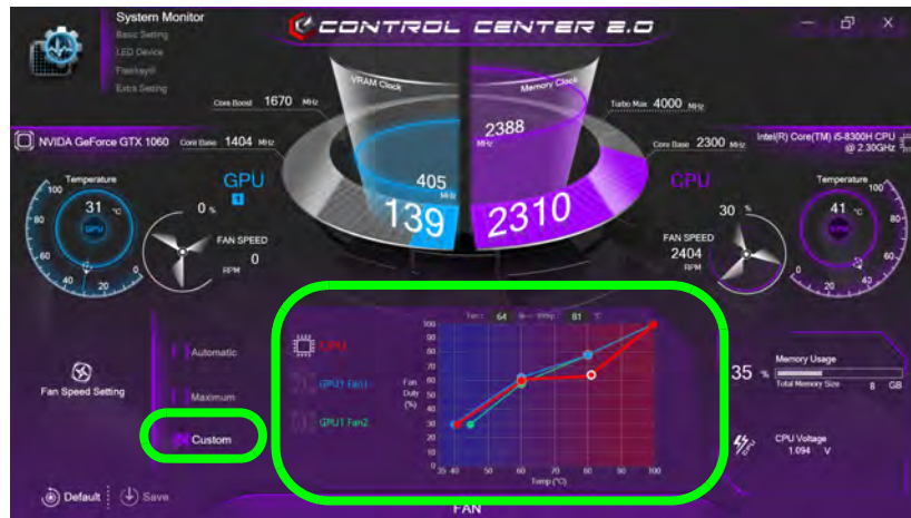
Figure B - 4 - CPU/GPU Fan Custom Settings
