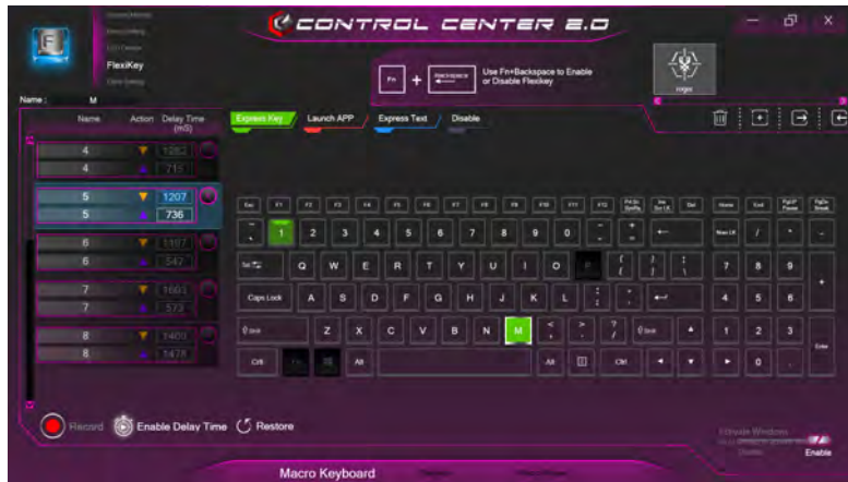
Figure B - 18 - Enable Delay Time
