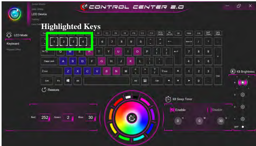
Figure B - 20 - LED Mode - Keyboard (Illuminated Color Per Key LED Keyboards))
