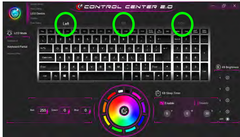
Figure B - 18 - LED Mode - Keyboard Partial (Illuminated Color LED Keyboards)
